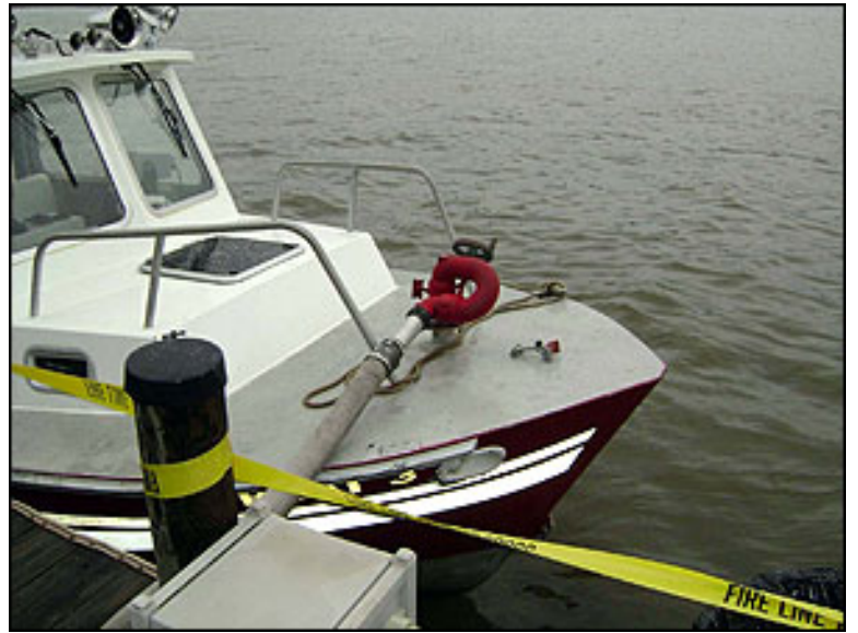
Solomon's Fire Boat 3 (750 gpm) pumps water using its bow monitor which is then relayed by the Clinton pumper to the fill point.
