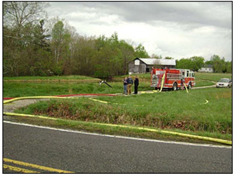
Fill Site #2 is operated by Charles County Engine 73 (1,500 gpm). They are drafting from a 6-inch dry fire hydrant using three, 10-ft sections of suction hose.
