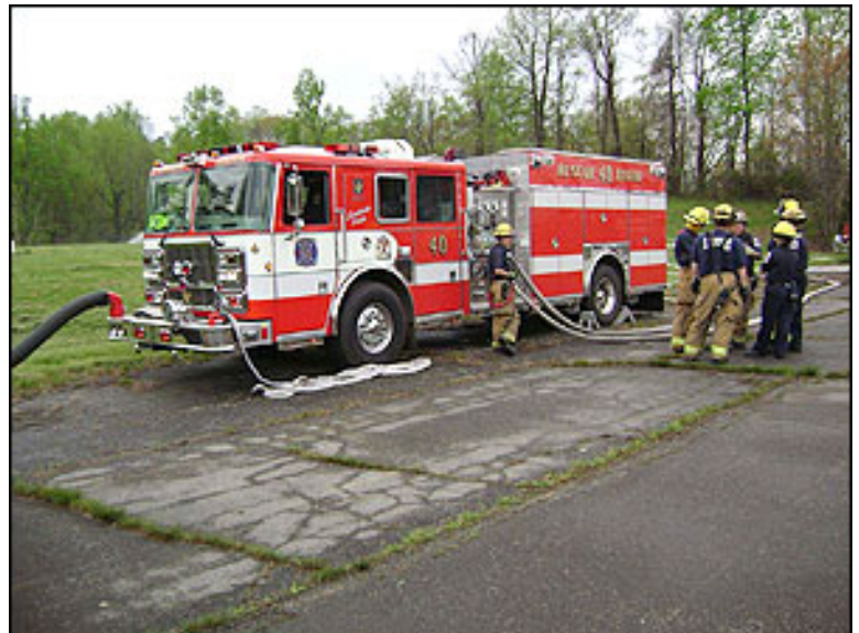
While awaiting the arrival of tankers, Brandywine VFD Rescue Engine 840 (1,500 gpm/500 gallon tank) begins to set-up a dump site while also pumping off its tanker water to E836B.
