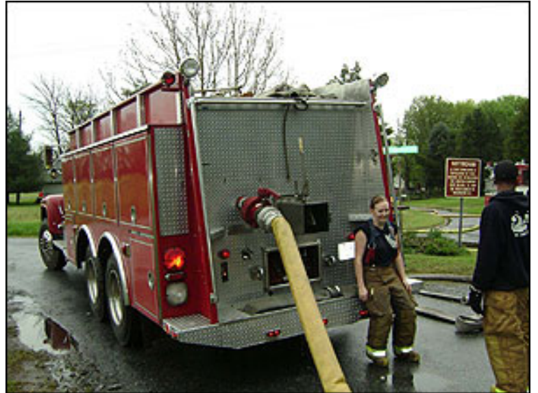
Fill Site #1 crews work to fill this tanker by using 5-inch hose in between torrential downpours of rain.
