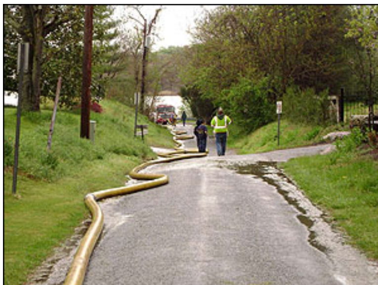
About 800 ft of 5-inch hose is used to supply the pumper at the dump tank.
