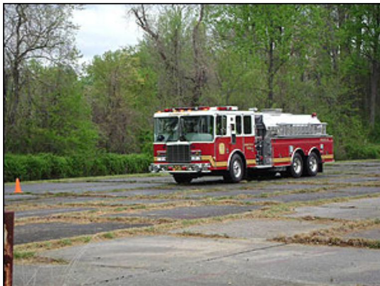
Forestville VFD Tanker 823 (2,500 gallon/1250 gpm) arrives very soon after Tanker 845 and begins to support the dump tank operation by off-loading its water into the dump tank.
