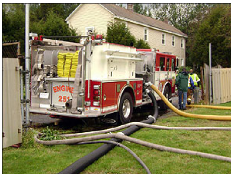
This Clinton pumper is drafting from the river to support the fill site.
