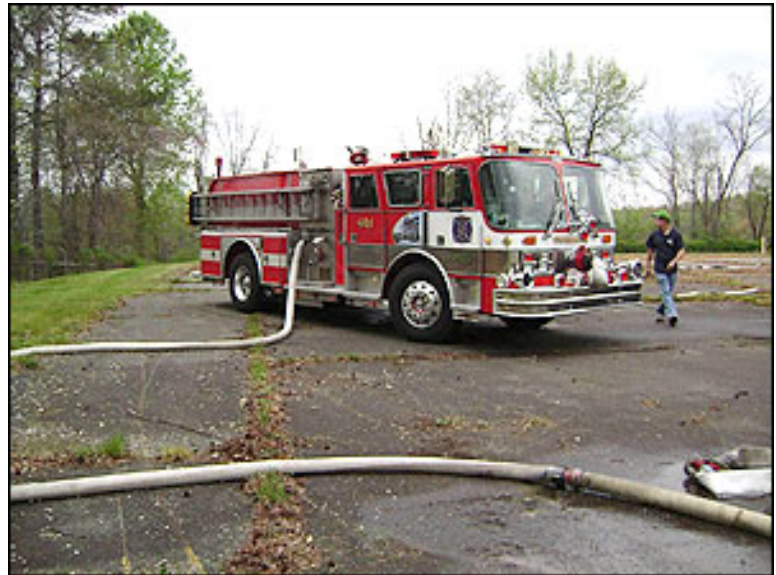
Brandywine Engine 840 (1,500 gpm/500 gallon tank) arrives and supports the fire attack by also pumping to E836B.
