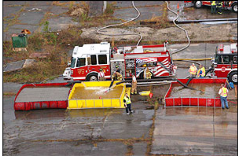
Denton Engine 304 establishes a second dump-site using three dump tanks. Note the roof ladder used to help spread out the tanks so that two, large tankers can get into position at the same time.
