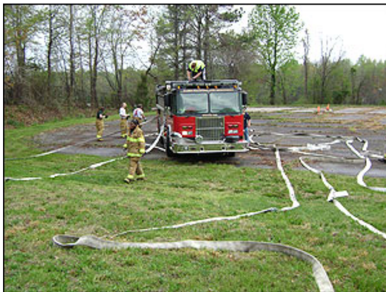
The drill begins with Baden VFD Engine 836B (1250 gpm/750 gallon tank) arriving on the scene and deploying a 1-3/4-inch attack line and getting supply lines into position.
