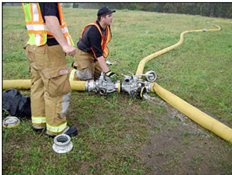
Two, LDH manifolds are used to supply the 5-inch hose for tanker fill lines. By using two manifolds, the 5-inch line can be drained much faster in between tanker fills.
