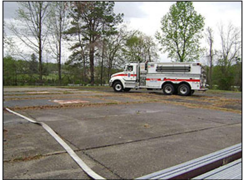
PGFD Tanker 845 (3000 gallon/1000 gpm) is the first tanker to arrive and moves into position to pump E836B's supply line. Due to a communications issue, the tanker was delayed in its arrival and the water flow at the attack line was interrupted for about 2-minutes.
