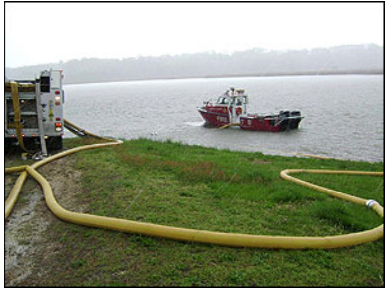
Charles Fire Boat 8 (750 gpm) drafts just off shore and supplies a 4-inch line.
