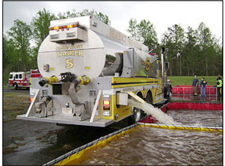
The flow is pushed to 500 gpm as more big tankers arrive to off-load water.
