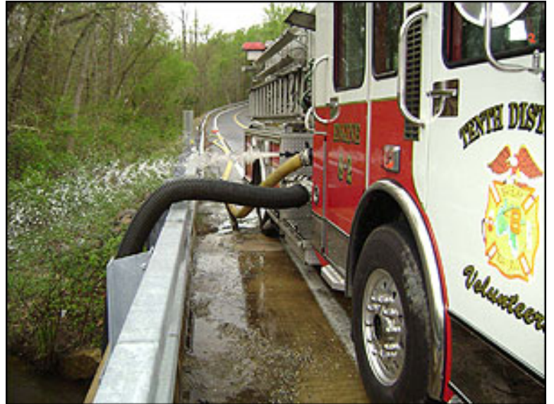
Marbury VFD E82 (2,000 gpm) operates at Fill Site #5 where they have to draft off of a bridge.
